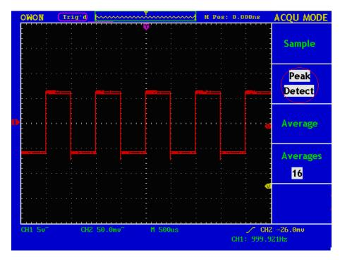
**Fig.5-28** Peak Detect mode, under which the burrs on the falling edge of the square wave, can be detected and the noise is heavy.
