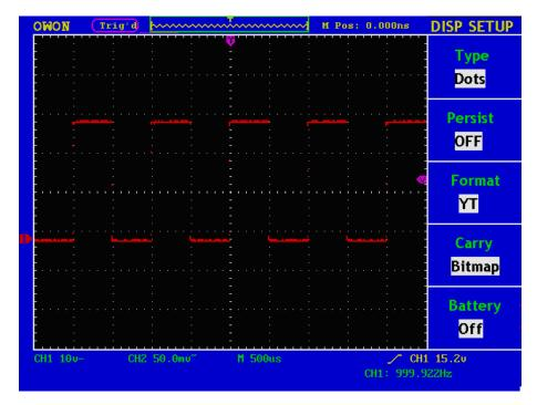
Fig.5-33 Display in Dots form
