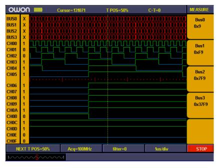
Fig.5-72: Bus measurement
