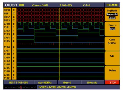
Fig.5-61: Sequential queue trigger
