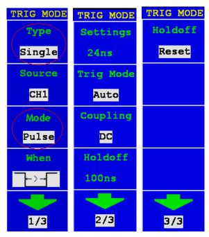
Fig. 5-21 Pulse Width Trigger menu
