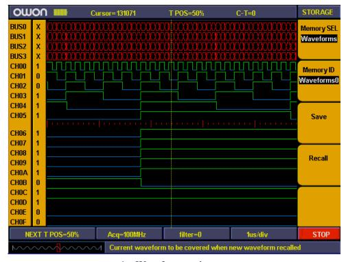
Fig.5-74: Waveform saving
