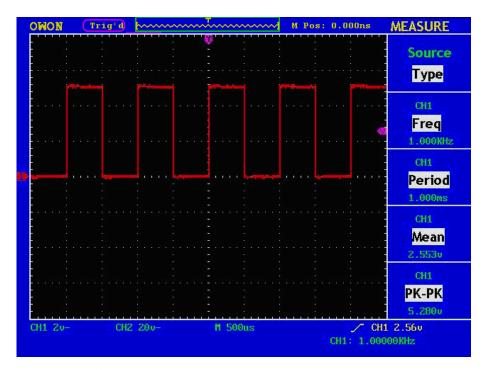
Fig.6-1 Waveform of Automation Measurement
