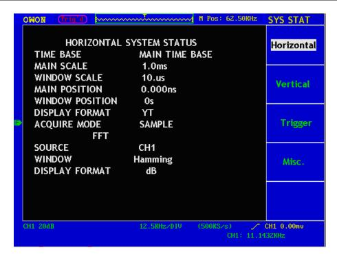
Fig.5-42 Horizontal System State
