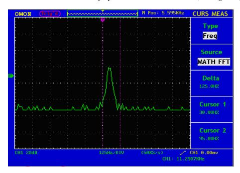
Fig.5-50 wave of Freq cursor measurement
