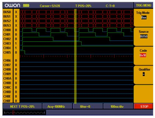
Fig.5-57: Bus trigger
