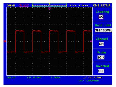
Fig. 5-2 AC Coupling Oscillogram
