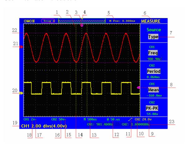
Fig. 4-3 Illustrative Drawing of Display Interfaces
