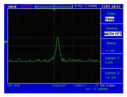
Fig.5-49 wave of Vamp cursor measurement
