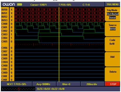
Fig.5-63: Distributed queue trigger
