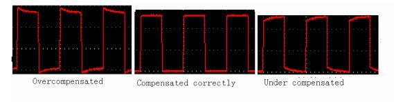
Fig. 4-5 Displayed Wave Forms of the Probe Compensation
