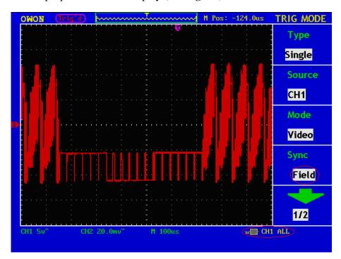
**Fig.6-7** Wave Form Obtained from Video Field Trigger
