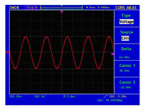
Fig.5-46 Waveform of Voltage Cursor Measurement
