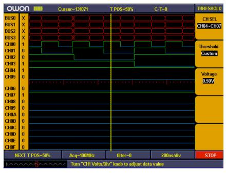
Fig.5-67: Threshold custom setting
