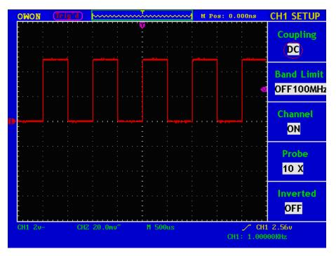
Fig. 5-3 DC Coupling Oscillogram
