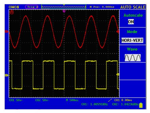
Fig.5-51: Autoscale Horizontal- Vertical multi-period waveforms
