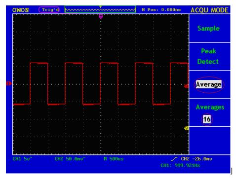
Fig.6-5 Wave Form of the Noise-Removed Signal
