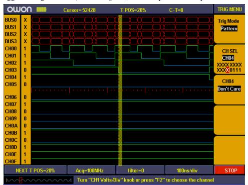
Fig.5-59: Pattern trigger
