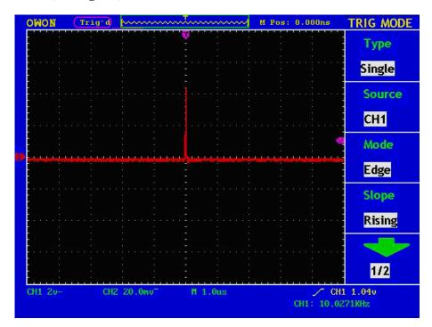
**Fig.6-3** Capture the Single Signal
