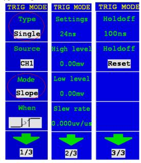
Fig.5-26 Alternate trigger(Trigger Type: Slope)Menu
