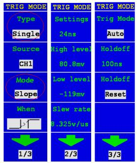
Fig. 5-22 Slope Trigger menu
