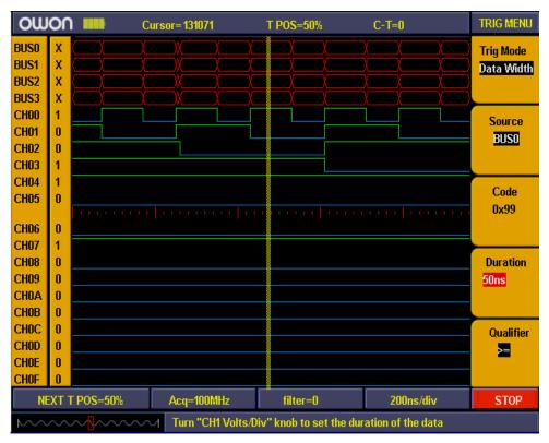
Fig.5-65: Data width trigger
