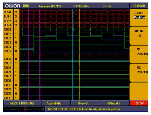
Fig.5-81: Cursor position measurement
