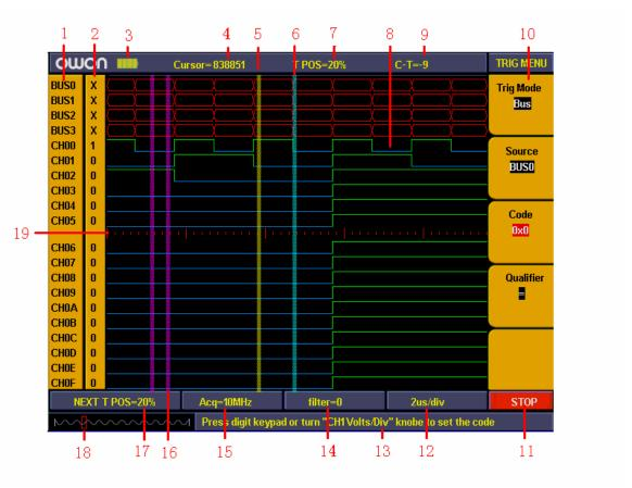
Fig.4-12: User interface of logic analyzer
