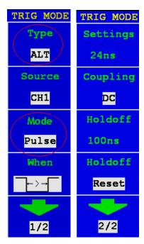
Fig.5-25 Alternate trigger (Trigger Type: Pulse) Menu
