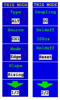
Fig.5-23 Alternate trigger(Trigger Type: Edge) Menu
