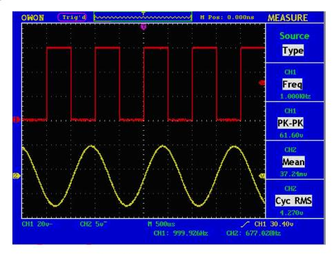
Fig.5-44 Automatic Measurement
