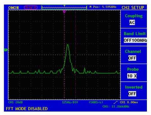
Fig. 5-4 Channel CH1 is disable under FFT mode
