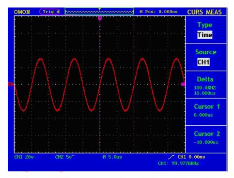
Fig.5-47 Wave Form of Cursor Measurement
